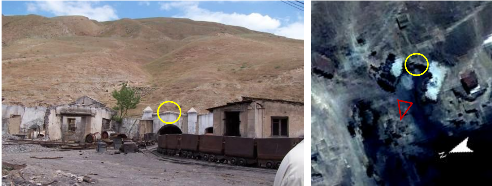
Figure 4: Photograph of an adit (left; yellow circle) and corresponding satellite view (right; yellow circle). The red triangle indicates angle of view of the photograph on the left.
