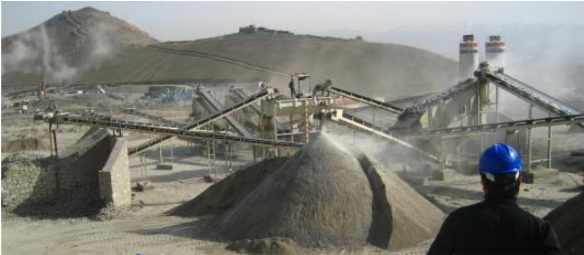
Figure 6: Photograph of one of the crushing and sorting plants shown on the satellite image on the right.
