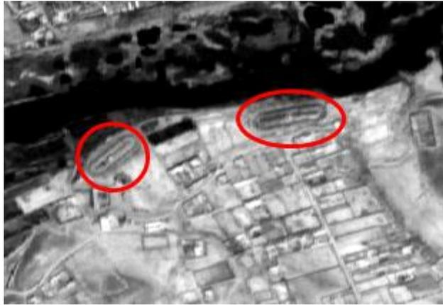
Figure 13: Typical river mining structures. The Bull's Trench kilns - marked in red - indicate that mining is for clay. Scale 1:10 000. Again two features are recognized by their context. The recognition of the river itself would not lead to the conclusion that clay pits exist, but the recognition of kilns at the shore of the river indicate the presence of clay pit activities.
